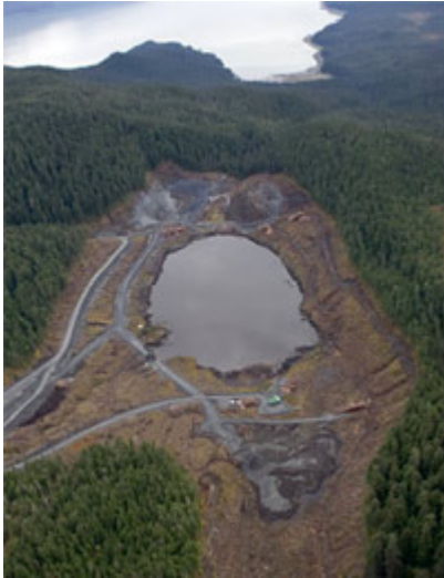
Lower Slate Lake, slurry disposal site for the Kensington Gold Mine (EarthJustice)
