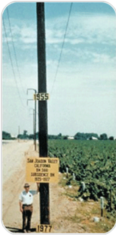
Picture showing land subsidence due to groundwater pumping in California Central Valley, 1977. (Photo courtesy of U.S. Geological Survey)
