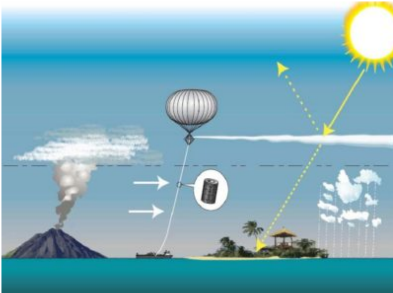
A tethered hose is another possible means to inject aerosols into the stratosphere.
