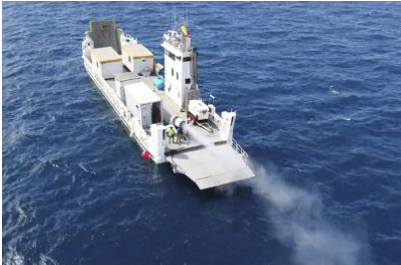
Testing marine cloud brightening equipment. Credit: Brendan Kelaher/Southern Cross University
